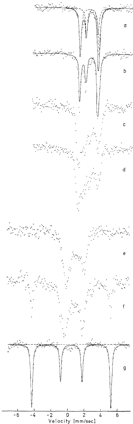
Fig. 5. Mössbauer spectra of \text{FeIz}_2 \cdot x \text{IzH} at room temperature after keeping the sample for 30 minutes in vacuum ( 10^{-4} Torr) at temperatures (a) 193 °C, (b) 201 °C, (c) 235 °C, (d) 242 °C, (e) 400 °C, (f) 461 °C, and (g) 505 °C. The solid curves in (a) and (b) correspond to \delta^{A,B} - and \Delta E_Q^{A,B} -values specified in Table 1 for the 300 K measurement. The solid line in (g) represents the \gamma\text{-Fe}_2\text{O}_3 spectrum with \delta = 0.453 \pm 0.008 mm sec ^{-1} , \Delta E_Q = 0.50 \pm 0.03 mm sec ^{-1} , and H^{\text{int}} = 508 \pm 2 kG. The outermost resonance lines in this magnetic spectrum are missing due to the relatively small velocity used in this series of measurement
